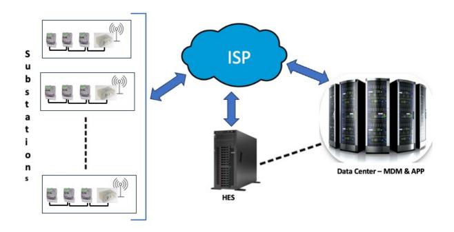
VData-09 is installed in a substation and is supplied with AMR Modem (4G), Power supply (redundancy - optional), CPU Card, Analog Input and output card (Optional), Digital Input and output card (Optional), Antenna, Power cable, communication cables, and other accessories.
